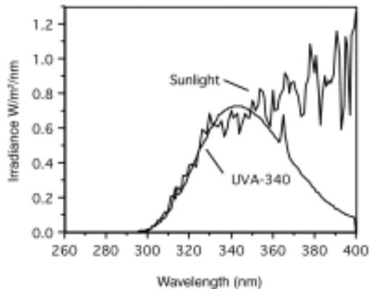
Fig. 3—Representative spectral power distribution, UVA-340 fluorescent lamps
